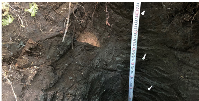
Photo 2. An example of a wetland soil pit with marks for each horizon.
